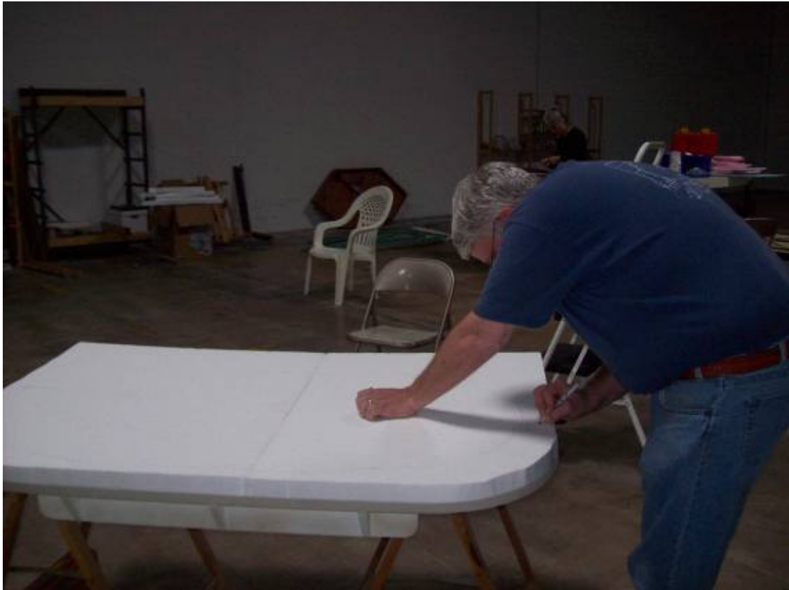
Photo 3. Ray Draws in the Track Centerlines
